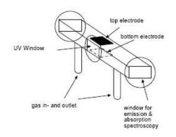
The Dielectric Barrier Discharge (DBD) cell.
