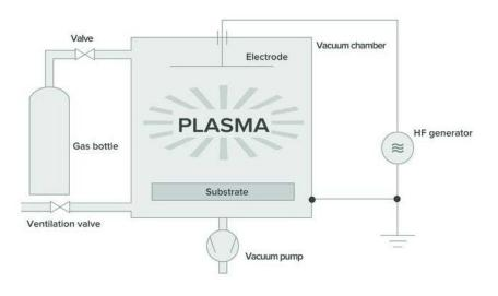
Plasma processing of silicon for semiconductor manufacturing.
