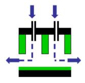
Hollow Pin Electrodes (Flow-Through)
