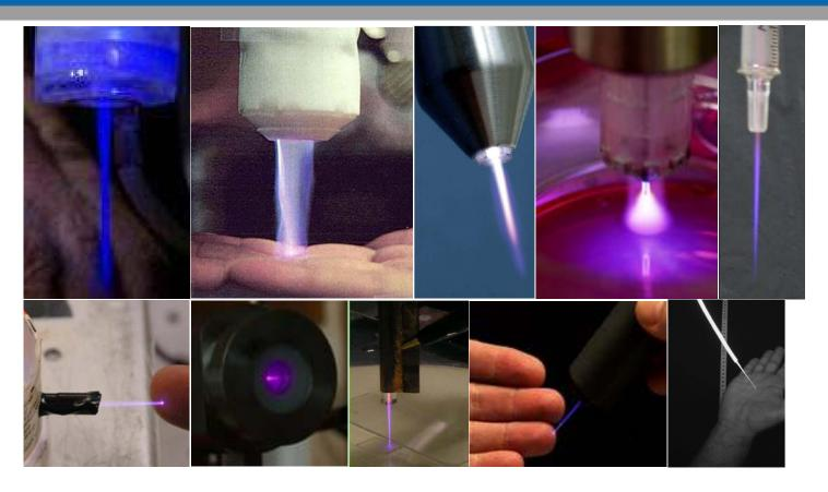
Gases used: Helium, Argon... or mixed with reactive gases  $(O_2, CH_4...)$
