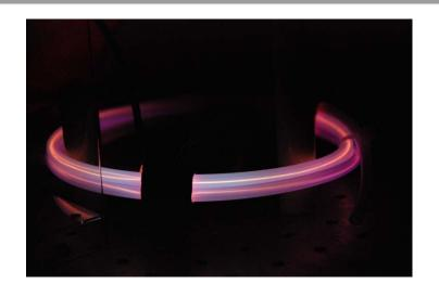
Distance the streamer can travel inside the insulating tubing depends on applied voltage, location of the powered electrode, type of working gas.
