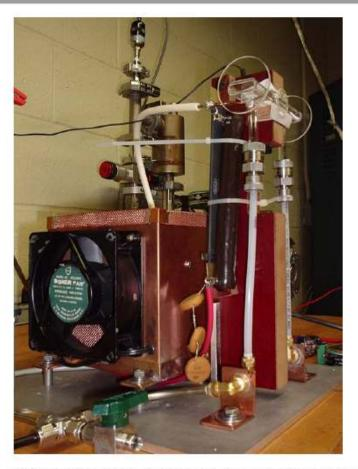
Side view of the DBD cell experiment with the fast high voltage transistor switch connected to the bottom electrode.
