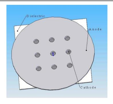
Parallel operation of multiple openings – *Multi-CBL structure*
