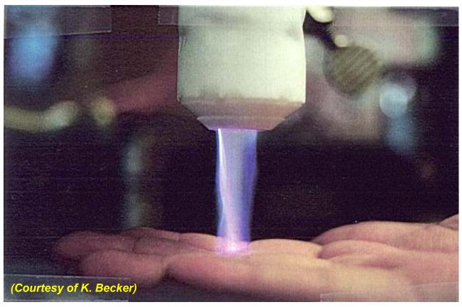
An Atmospheric Pressure Plasma Generated with a Capillary-Plasma-Electrode Discharge
