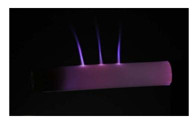
Pure helium (8 slm); Teflon tube (OD=½"; ID=¼") 3 holes (diameter: 1/16") on side wall
